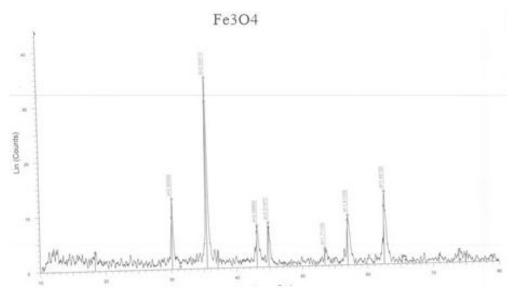
**Fig.2.** XRD pattern of *Fe3O4* monocrystalline.
