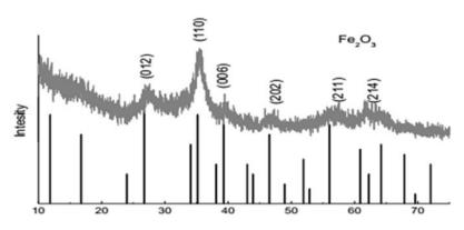
Fig.1. XRD pattern of Fe2O3 nanocrystalline sample
